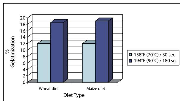
Figure 5 clearly shows that increased conditioning time and temperature increases gelatinization in feed, regardless of the cereal base used. The process of gelatinization creates natural 'glues' which allow the feed particles to compress tightly and adhere to each other when passing through the pellet die. Optimal 'cooking' of feed will result in more durable pellets and reduce levels of fines (Figure 6).
