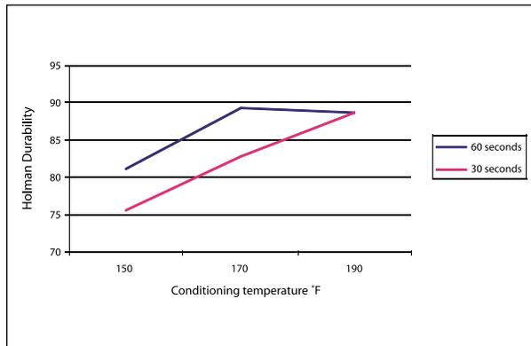
As the conditioning time and temperature was increased, the pellet durability increased (as expressed by a Holmen Durability Index).
