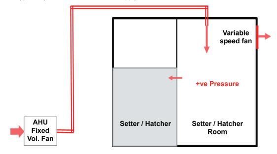
Figure 2: Typical layout of a fixed volume air supply room.
