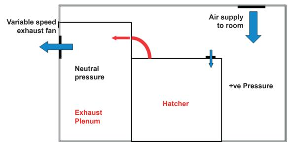
**Figure 13:** In this example, a sharp elbow is used as the top exit exhaust of the hatcher into the exhaust plenum. The sharp 90° change in direction can cause back pressure on the exhaust of the hatcher.
