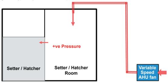
Figure 4: Typical layout of a variable speed air unit.
