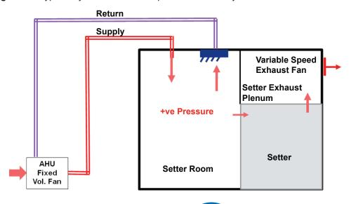
Figure 10: Typical layout of an exhaust pressure control system.
