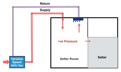
Figure 6: Typical layout of a fixed volume air supply with return air unit.
