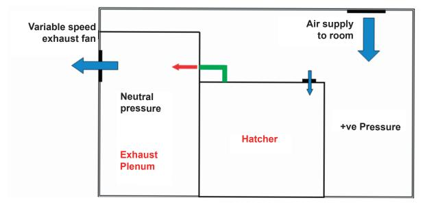
The configuration in **Figure 14** should also be avoided. It may result in back pressure on the exhaust of the hatcher since it is trying to make the hot air from the hatcher go up and then down into the plenum. This works against the natural tendency of hot air to always try to go upward.
