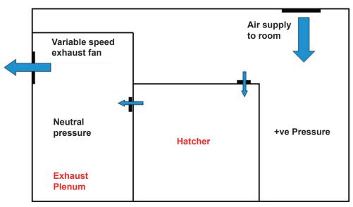
Figure 11: A typical configuration of the hatcher and plenum.
