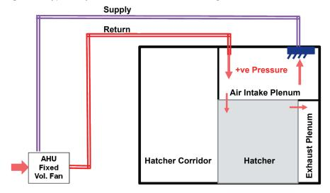
Figure 7: Typical layout of fixed volume air handling unit with air return for hatchers.
